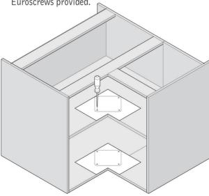
3 Using a bradawl mark the position of the fixing holes, then using a drill and 5 mm drill bit drill the fixing holes to a depth of 15 mm.
