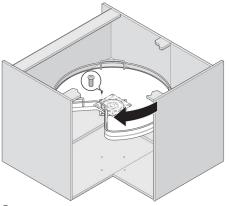
5 Line up the fixing holes with the bottom plate of the turntable as shown above, fix the first hole using 1 x 6.3 x 14 mm Euroscrew.
