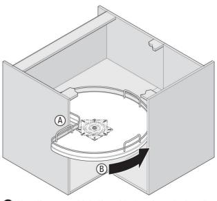
4 Place the carousel into the cabinet as shown in steps A and B above.
