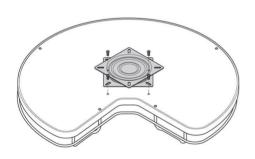
2 Position the drilling template on the desired shelf in the cabinet as shown above.
