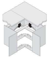
Fit worktops once the cabinet has been secured into place. If the carousel has been retro fitted into an existing cabinet, worktops will already have been fitted.
