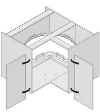
Fix the cabinet doors to the cabinet. If the carousel has been retro fitted into an existing cabinet, doors will already have been fitted.
