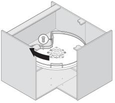
$\mbox{\Large 6}$  Carefully turn the crousel clockwise through 90  $^{\circ}$  making sure the bottom plate of the turntable stays in position, fix the next hole using 1 x 6.3 x 14 mm Euroscrew.
